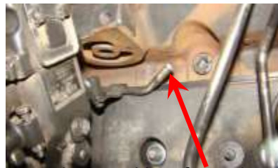
End of steel line from the P-7100 that connects to the tank return line. Figure 34
