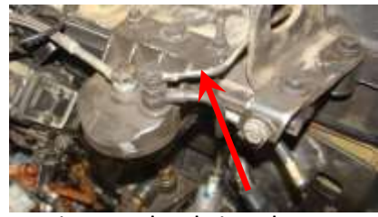
Injector Bleed Line that connects to the tank return line. Figure 35
