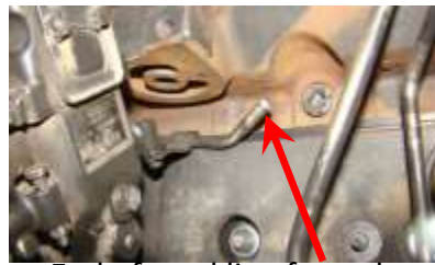
End of steel line from the P-7100 that connects to the tank return line. Figure 54
