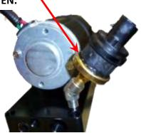
**NOTE:** IF THIS KIT IS BEING USED FOR AN AirDog®II-4G, REMOVE THE PIPE PLUG FROM THE 90° FITTING ALREADY INSTALLED ON THE PUMP AND INSTALL THE PRESSURE SWITCH IN THAT FITTING. THE 45° FITTING IS NOT USED.
