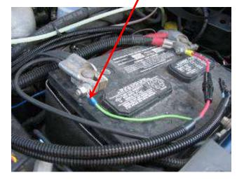
3. Find a key on hot wire to install the wire tap onto. A good source is the cigarette lighter port positive wire.
