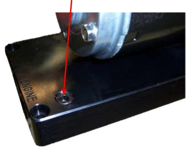
2. Install the 45° elbow (4A-5-02-02S) in the port. Be sure face it away from the motor. **DO**
