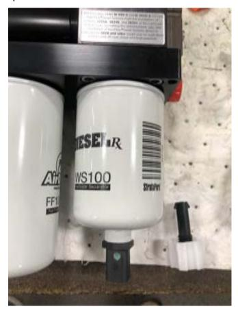
2-4. Once the new filter is installed, remove the previously installed hose clamps and key the truck on/bump the starter depending on what application of truck it is to prime the fuel system. Propery dispose of the waste fuel that was caught by the bucket or pan used.
