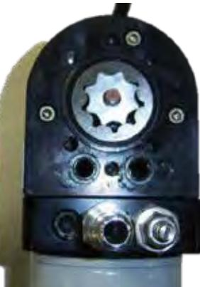
**STEP 8:** Loosen assemble the cap screws. Torque the cap screws in an opposing pattern.
