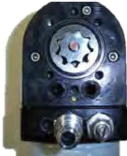
**STEP 3:** Remove and clean the Gerotor. Be very careful to not damage the Gerotor.
