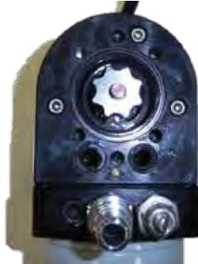
**STEP 6:** Align and install the outer gear and O-rings.
