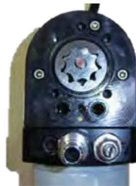
**STEP 7:** Install the Gerotor Cap. Be very careful not to dislodge or pinch the O-rings.
