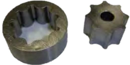
**STEP 4:** Remove the O-rings and clean/inspect the inside of the Gerotor pocket.
