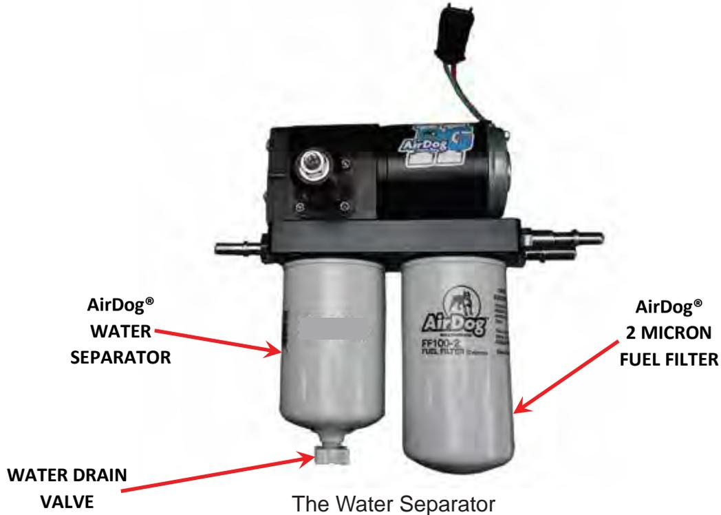
Replace the water separator every other time you change the Fuel Filter or if it becomes damaged or plugged. It is suggested to check/drain the water separator every three months or as needed should you experience excessive 'water in fuel' conditions. When installing the water separator, be sure to clean the underside of the AirDog® base. Follow the instructions printed on the pre-filter for proper tightening procedures.
