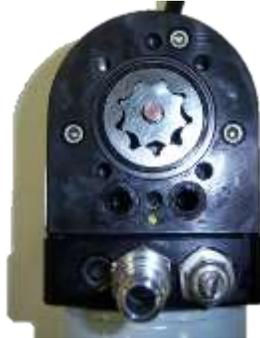
**STEP 3:** Remove and clean the Gerotor. Be very careful to not damage the Gerotor.
