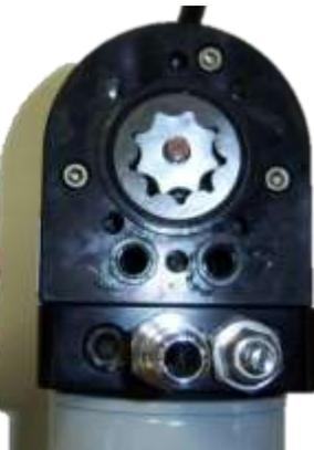
**STEP 8:** Loose assemble the cap screws. Torque the cap screws in an opposing pattern.
