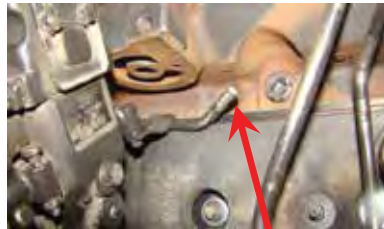
Figure 57 End of steel line from the P-7100 that connects to the tank return line.
