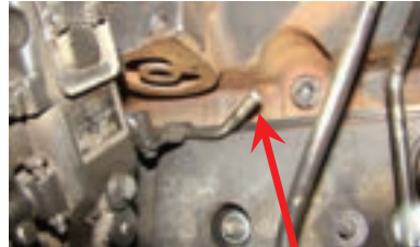
Figure 47 End of steel line from the P-7100 that connects to the tank return line.
