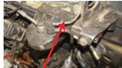
Figure 58 Injector Bleed Line that connects to the tank return line.
