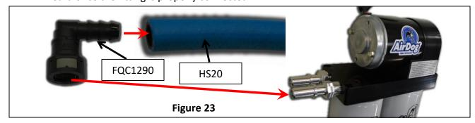
6B-4. Run the fuel line along the frame as mentioned in step 5-3 to the filler neck tee. Cut the fuel line to length and insert fuel line end FQC12S per step 5-1. Once the connector is installed, connect it to the male J2044 fitting in the filler neck tee (001-4A-1-0150). A "click" will be heard once properly connected.
