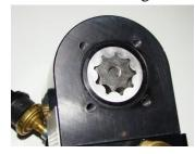
Step 7 Install the gearotor cap. Be very careful to index the cap to position the wide space between the half moon cuts to the bottom.
