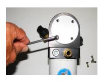
Step 4 Clean the inside of the gearotor pocket.
