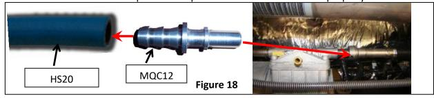
6A-3. Run the other end of the fuel line along the frame as mentioned in step 5-3 to the "Engine" port in the AirDog®. Cut the fuel line to length and insert fuel line end FQC12S per step 5-1. Once the connector is installed, connect it to the male J2044 fitting in the "Engine" port in the AirDog®. A "click" will be heard once properly connected.
