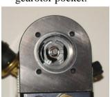
Step 5 Replace the O'ring and center gear.
