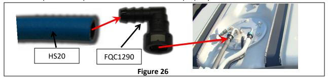
6C-3. Run the fuel line along the frame as mentioned in step 5-3 to the AirDog® "Fuel In" port. Cut the fuel line to length and insert fuel line end FQC12S per step 5-1. Once the fuel line end is pressed in, connect it to the male J2044 fitting in the AirDog® "Fuel In" port. A "click" will be heard once properly connected.
