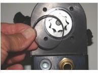
Step 5 Replace the O'ring and center gear.
