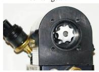
Step 8 Replace the cap into position. Be very careful, do not pinch the O'ring. Torque the cap screws. in an opposing pattern.
