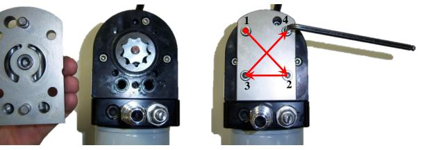
If there is damaged found to either the Gerotor, Gerotor pocket, or O-rings, call into AirDog® Tech Support for further assistance.
