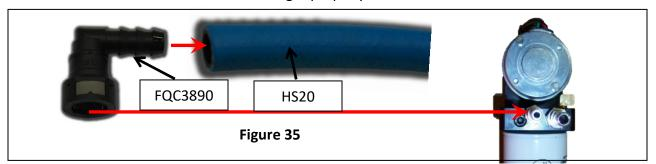
6C-4. Run the fuel line along the frame as mentioned in step 5-3 to the filler neck tee. Cut the fuel line to length and insert fuel line end FQC12S per step 5-1. Once the connector is installed, connect it to the male J2044 fitting in the filler neck tee (001-4A-1-0175). A "click" will be heard once properly connected.
