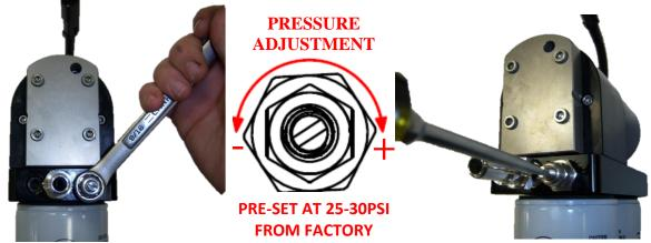
Turn the adjuster screw counter-clockwise to reduce the output
