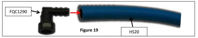
6A-4. Run the fuel line along the frame as mentioned in step 5-3 to the "Engine" port in the AirDog<sup>®</sup>. Cut the fuel line to length and insert fuel line end FQC12S per step 5-1. Once the connector is installed, connect it to the male J2044 fitting in the "Engine" port in the AirDog<sup>®</sup>. A "click" will be heard once properly connected.
