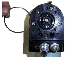
**STEP 7:** Install the Gerotor Cap. Be very careful not to dislodge or pinch the O-rings.
