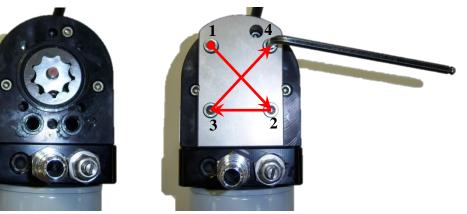
If there is damaged found to either the Gerotor, Gerotor pocket, or O-rings, call into AirDog® Tech Support for further assistance.
