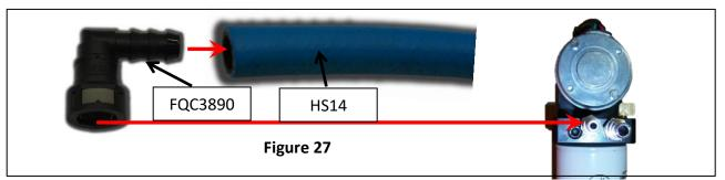
6C-4. Run the fuel line along the frame as mentioned in step 5-3 to the filler neck tee. Cut the fuel line to length and insert fuel line end FQC12S per step 5-1. Once the connector is installed, connect it to the male J2044 fitting in the filler neck tee (001-4A-1-0200). A "click" will be heard once properly connected.
