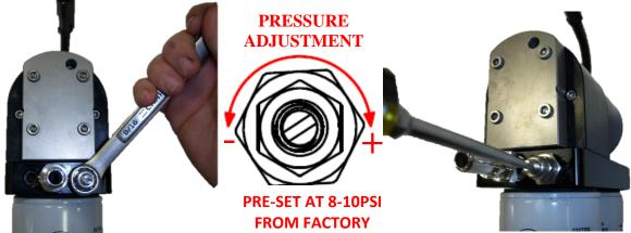
Turn the adjuster screw counter-clockwise to reduce the output pressure
