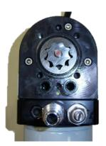
**STEP 8:** Loose assemble the cap screws. Torque the cap screws in an opposing pattern.
