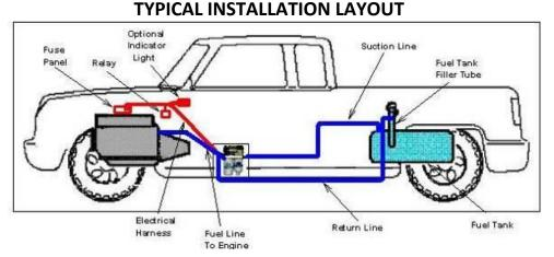
The AirDog<sup>®</sup>II-4G draws fuel from the fuel tank at a constant flow, removing water, particulates, and air/vapor. A regulated pressurized flow is maintained to meet the engine's varying fuel demands. The separated air/vapor and excess fuel not needed by the engine are returned from the AirDog<sup>®</sup> to the fuel tank.
